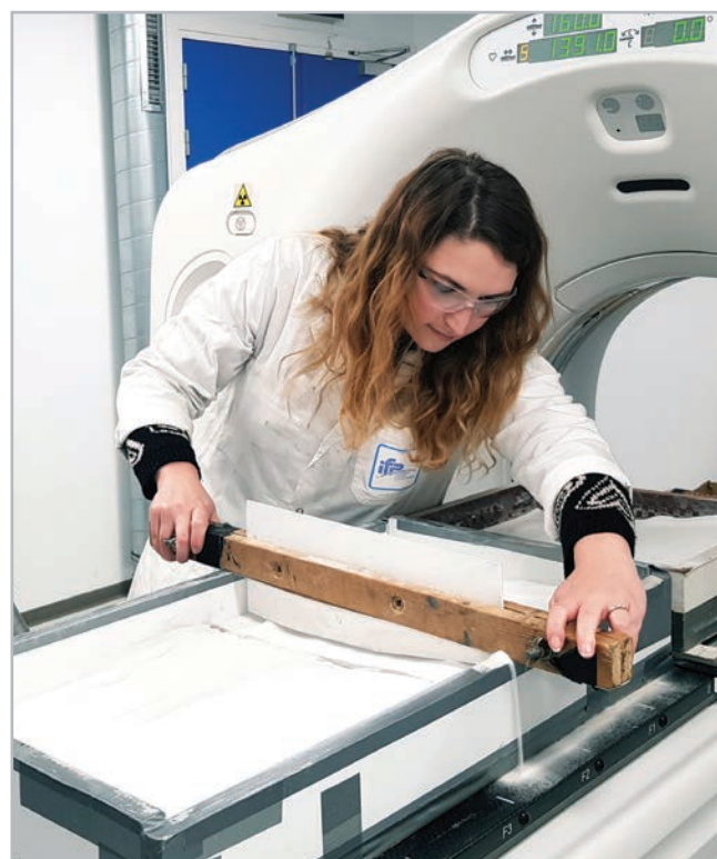
Analogue modelling in action: applying additional sand layers at certain time intervals during model runs (left), and ensuring even distribution of sand layers (right)
