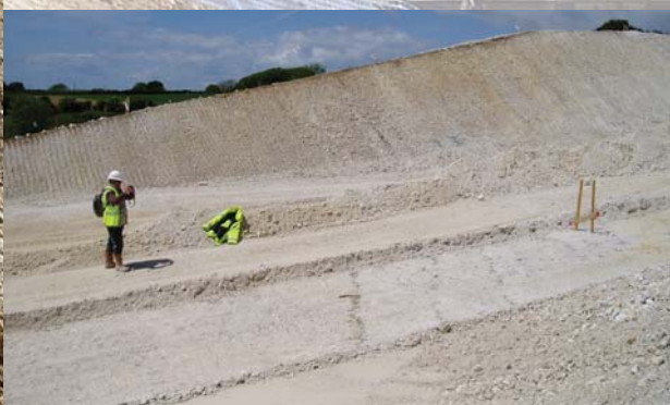
Rory Mortimore records the positions of three steeply dipping flint bands in the Seaford Chalk Formation
